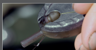
2 Next place the Rubber Quick Bead through the same hole in the base.
