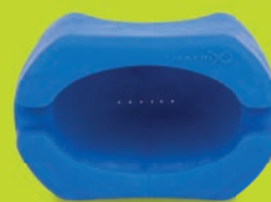
The small holes in the base of the mould prevent a vacuum forming during compression producing a better loading
